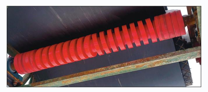
The Clean Weave Return Roll is comprised of polyurethane discs which offer abrasion resistance and wear life at least 5X longer than steel or rubber rolls.
