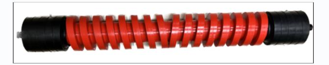
The Clean Weave Return Roll consists of polyurethane discs that provide exceptional resistance to abrasion and a wear lifespan at least five times greater than that of steel or rubber rolls.
