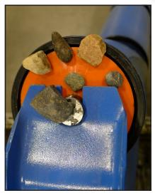
**Stationary Disc Design:** A durable polymer disc is seated inside the end cap and remains stationary as the roller rotates around it, preventing seizing even with material buildup between the roller and idler frame. Made from flexible, impact-resistant polymers, the seal is easily installed on-site with minimal downtime.
